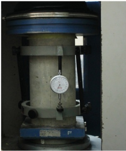
FIGURE 4: Compressive strength and modulus of elasticity test setup.
